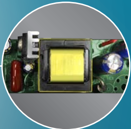
IC DRIVER Driver independiente multivoltaje AC100-240V
